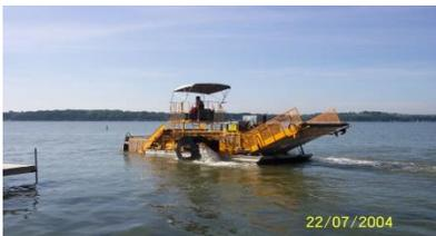
The Shore barges are Orange. They are out every day and there are typically 2 or 3 staff working with them (see photo below). They pick up floating aquatic plants in and around the shores that have floated in. These machines are not used for pile pick up.
