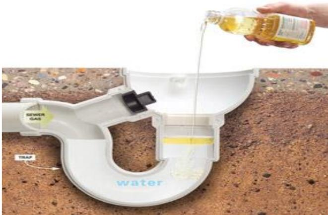
The term “sewer gas” is generally used in describing the odor people smell if a trap dries out. The actual gas may be made up of a number of different components, some of which may be hazardous.
